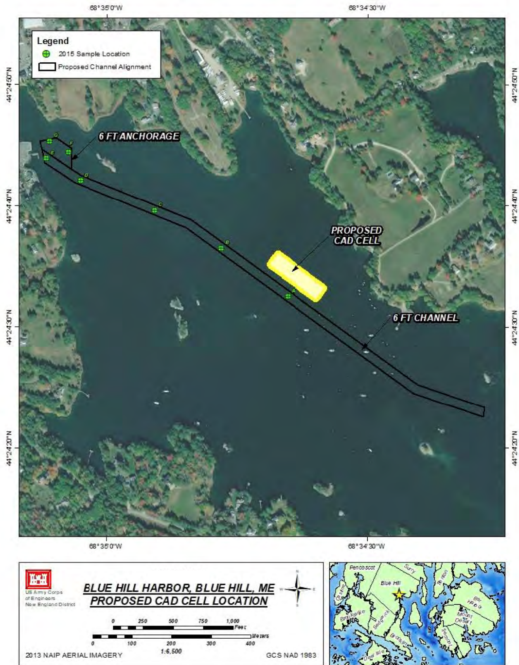
Figure 4: Blue Hill Harbor Confined Aquatic Disposal (CAD) Cell.
